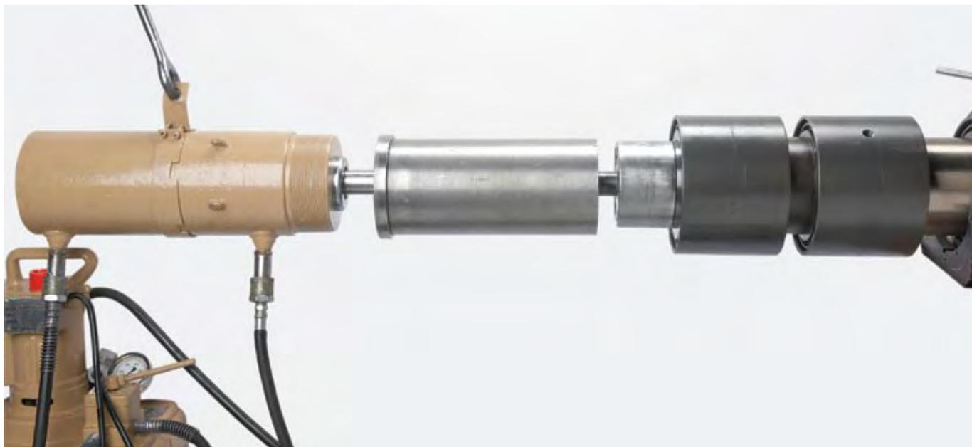
Fig. 28 Tooling used to push bearing onto shaft
