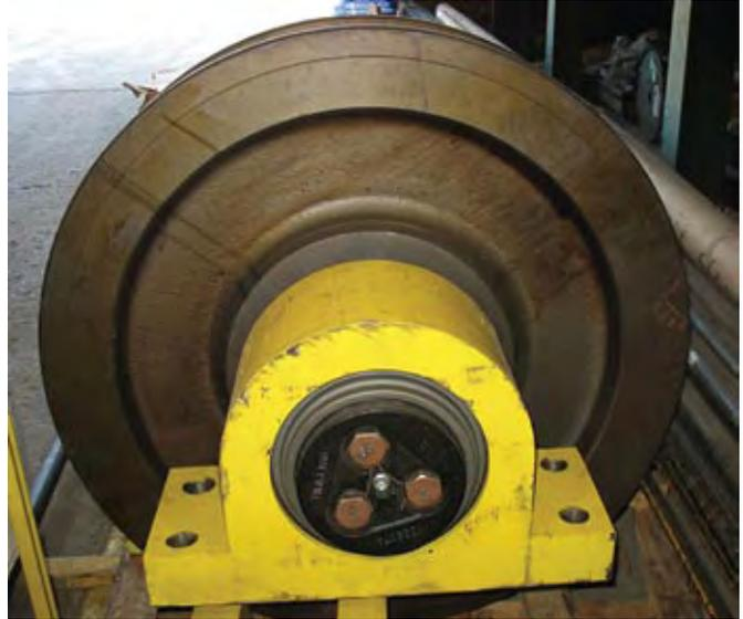
Fig. 12 AP bearings used in pillow block application
