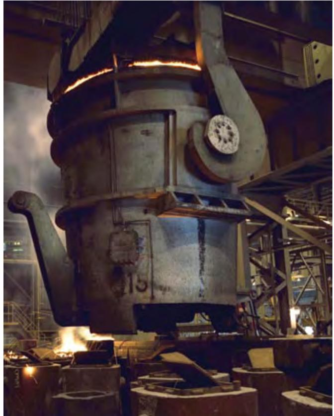
Fig. 17 Bottom pour ingot car equipped with Timken AP bearings
