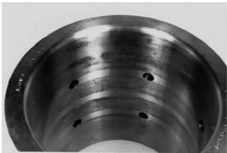
Fig. 7 Fretting ( Outer ring raceway surface )
