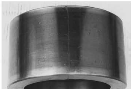
Fig. 3 Cracking ( Outer ring )
