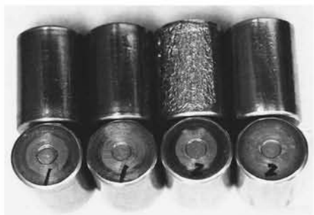
Fig. 2 Flaking ( Rolling contact surface of rollers )
