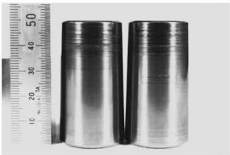
Fig. 8 Smearing ( Rolling contact surface of rollers )
