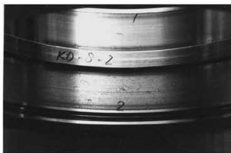
Fig. 13 Brinelling ( Outer ring raceway surface )
