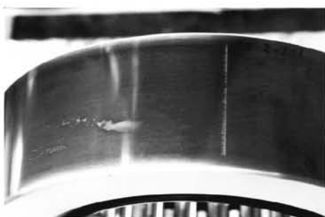
Fig. 12 Brinelling ( Outer ring outside diameter surface )
