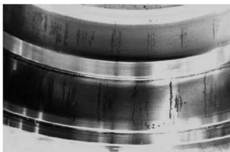
Fig. 11 Rust and Corrosion ( Outer ring raceway surface )
