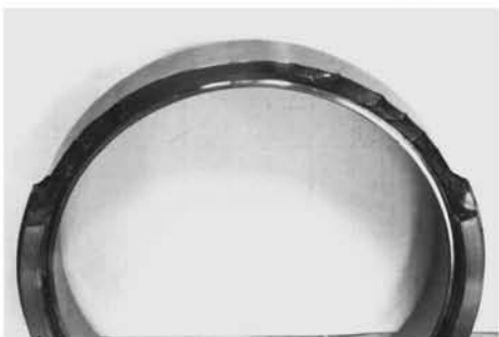
Fig. 5 Chipping ( Outer ring )
