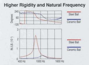
**FIG. 5:** Dynamic stiffness analysis performed before/after grinding spindle rebuilding shows higher rigidity and higher natural frequency for hybrid bearings, making them less sensitive to vibration.
