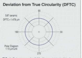
FIG. 1: Polar trace of a 5/8" silicon nitride ball indicates near perfect roundness, a characteristic which results in dramatically lower vibration levels.
