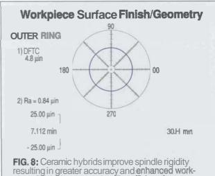
resulting in greater accuracy and enhanced workpiece finish characteristics, Form Talysuff traces show high degree of precision in finished part.
