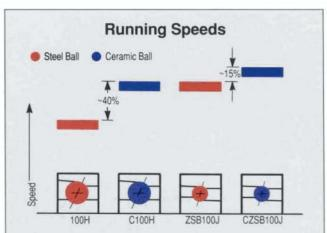
FIG. 3: Running speed of large diameter ceramic ball exceeds same-size steel ball by 40%. Converting to a small diameter ceramic ball will boost running speeds an additional 15%.
