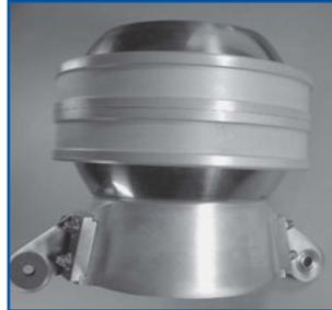
**5.** Main Rotor Swashplate Slider Bearings
