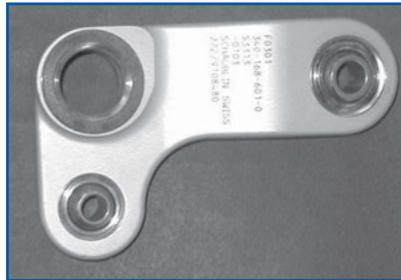
**8.** Thrust Reverser Linkage Bearings
