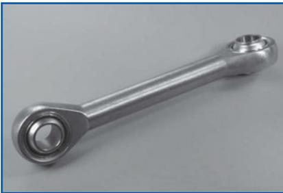
**2.** Tail Rotor Pitch Link Bearings
