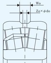
Note: See the dimension table for information on the oil groove width W<sub>o</sub> and oil inlet diameter  $\phi$  d<sub>o</sub>.
