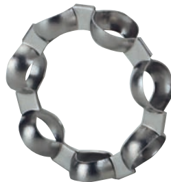
myonic type "48" loosely crimped two piece ribbon cage for low torque
