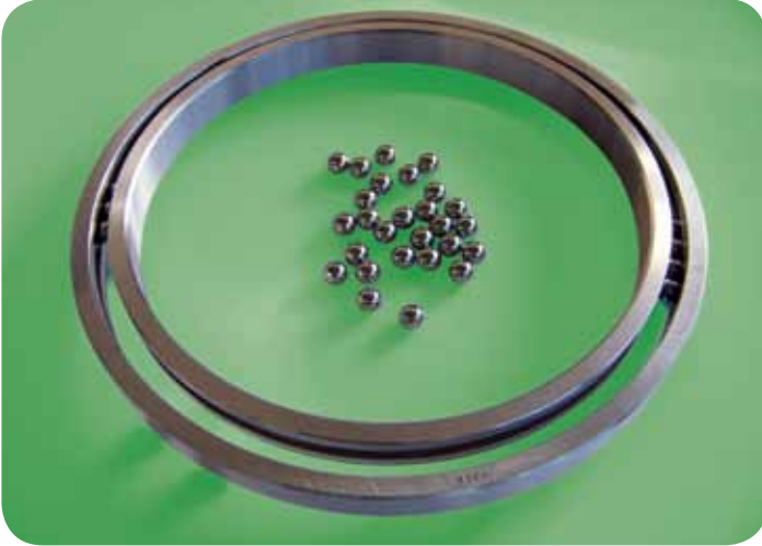
Filling of the bearing
