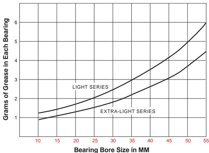
Figure 17 – Grease Quantity Chart
