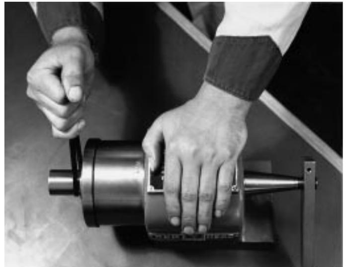
Figure 7 – Tightening with Spanner Wrench
