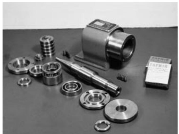
Figure 3 – Wheelhead Parts
