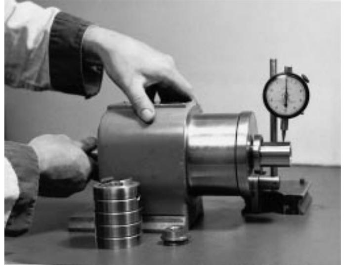
Figure 6 – Checking Nose-End Runout
