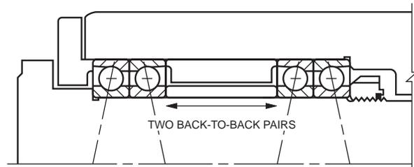
Figure 7 – DB-DB Mounting, Fixed (Not Recommended)
