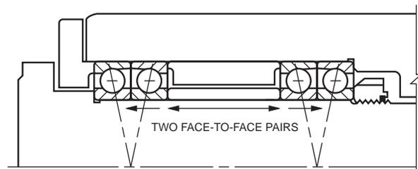
Figure 8 – DF-DF Mounting, Fixed (Not Recommended)
