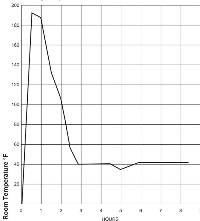
Typical Temperature After Break-In Procedure
