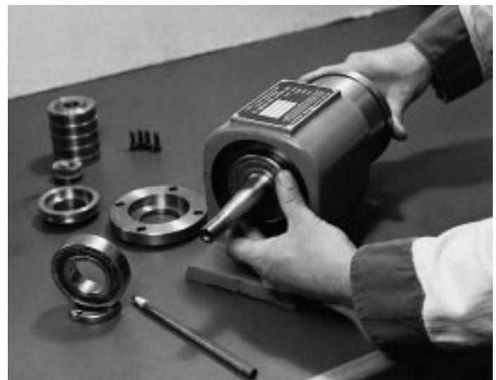
FIGURE 5 – MOUNTING DRIVE-END BEARINGS
