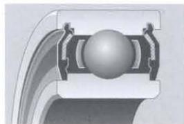
**Barseal™** is a composite seal consisting of molded rubber with a metal stiffener. It offers optimum sealing and is designed to contact the inner ring intimately under all loading conditions. The inner ring seal riding surfaces are ground for better sealing, lower torque and longer life.
