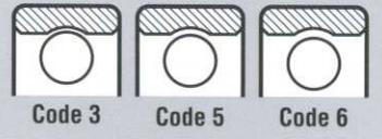
Specifying a radial play code must take into account the installation practice. If a bearing is press-fit onto a shaft or into a housing, its radial internal clearance is reduced by approximately 80% of the interference fit. Thus, an interference fit of .00025" would cause a .0002" decrease in internal clearance.
